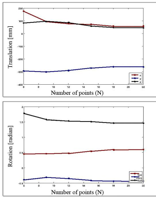
Fig. 7. Evolution of the rotation and translation matrices estimates by the calibration method according to the number of points used in the approach.
