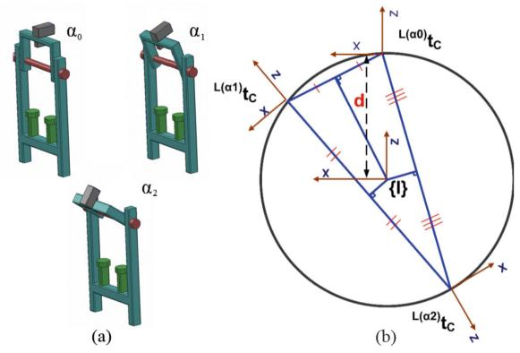
Fig. 2. a) The proposed approach uses different laser acquisitions in three different planes, which are estimate using the inertial sensor ( $\alpha_0$ ,  $\alpha_1$  and  $\alpha_2$ ); and b) The circumcircle of  $\triangle {}^W P^{\alpha_0} {}^W P^{\alpha_1} {}^W P^{\alpha_2}$  (shown in a perpendicular view to the X-Z plane of  $\{I\}$  which contains the triangle).
