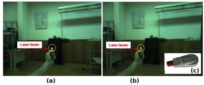
Fig. 6. a) and (b) Real example (left and right images) for one step in collecting some correspondence points by stereo camera and tilt-LRF with the  $\alpha = 23.2^\circ$ ; and (c) A simple laser pointer with a red-color plastic is the only calibration object; and b) .
