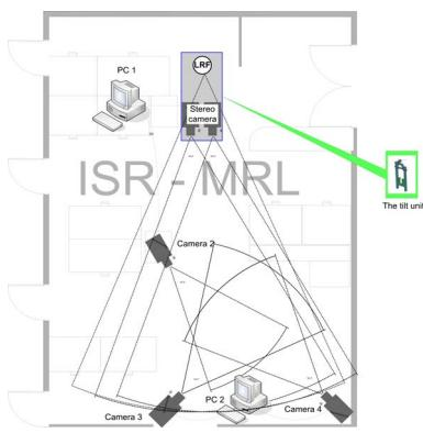
Fig. 3. The infrastructure of a multi-modal sensor network.
